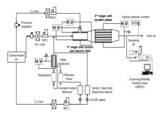
Figure 1. Experimental set up in this study.
