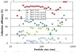
Figure 2. Size-dependent collection efficiency of the ESP with change of applied voltage between upper and bottom plates.
